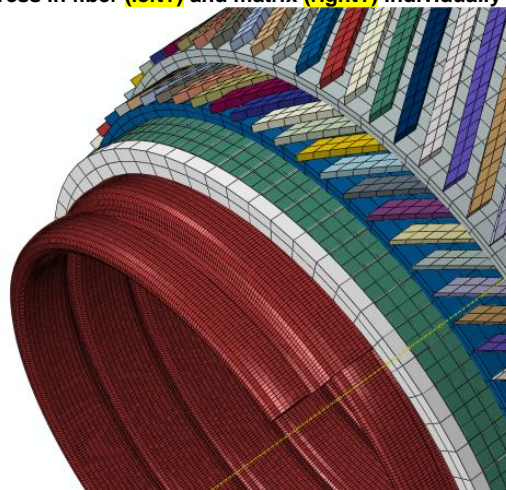
Figure 4. Finite element model used to study composite - metallic layer interactions
